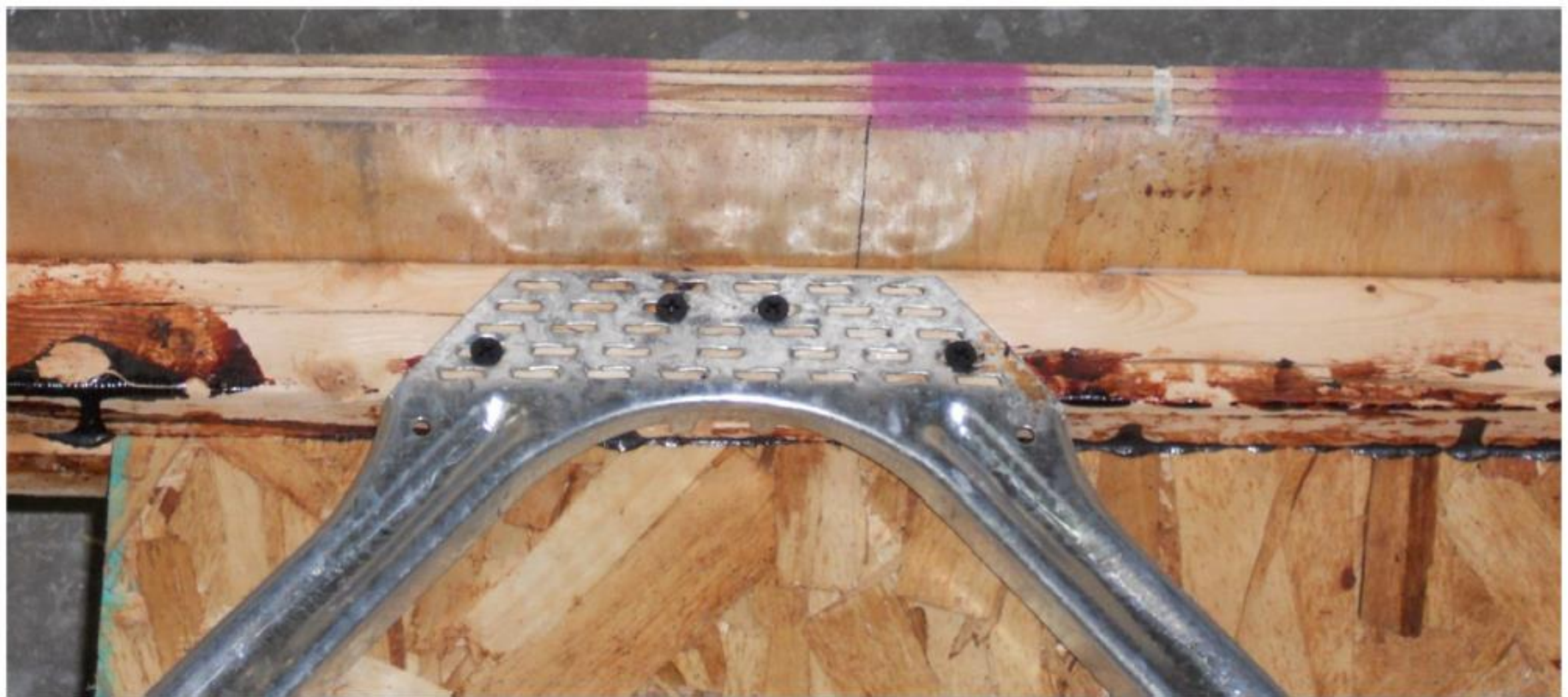
Figure B-13: Steel/wood connection in hybrid joist (H3) reinforced with screws
